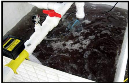
**One half quart of motor oil and cinder clay** was added to the holding tank and re-circulated with the centrifugal pump to maintain the oil and clay in suspension.
