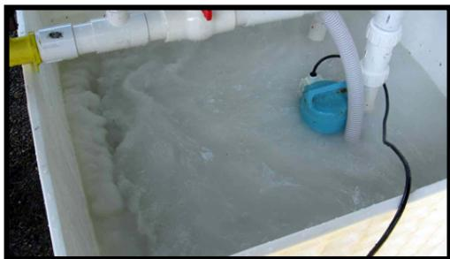
The test was conducted using two 360 gallon open top storage bins. One used as a sediment holding vault, the other as a receiving vessel. A channel connecting the two bins held the VMS. The VMS was connected to a two-inch hose with an in-line turbine flow meter and pressure gauge. The assembly was connected to a 110 gpm submersible centrifugal pump.
