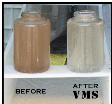
**Conclusion:** The VMS had the ability to remove the 2270 Mg/L oil in the sediment-laden water to non-detectable levels and no oil sheen was visible in the receiving vessel for the duration of the test.
