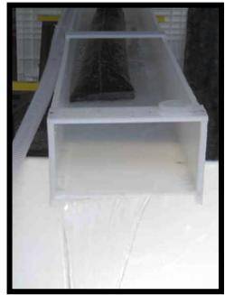
**samples were taken from the outfall channel** after filtering thru the VMS. The flow rate during this test maintained a flow rate above 30 GPM with a pressure of 3.0 PSI. The VMS retained over 5 pounds of sediment during the test.
